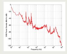
The phase noise linear spectral density of the laser.
