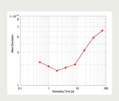
The Allan deviation of a Stable Laser Systems integrated frequency-stabilized laser system, as measured by heterodyning against a more stable system. Hertz-level linewidths are realized. Exact performance may differ due to natural variability in the thermal noise of mirror coatings.
